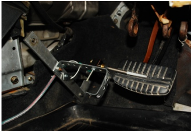
Fig.3. Micro switch at brake pedal
