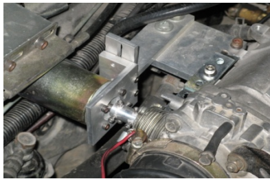
Fig.4. Drive-by-wire throttle valve system
