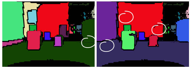
(c) Graph segments with only color difference as a cluster criterion. (d) Graph segments with only surface normals as a cluster criterion.
