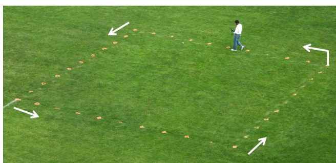
Fig. 10. Calibration step points around the square calibration loop.
