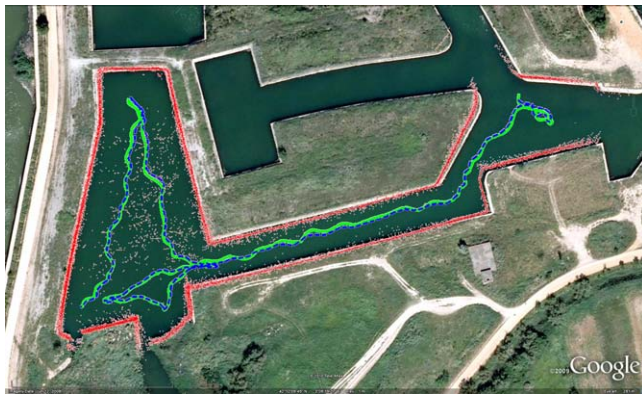
Fig. 6. Trajectory and map estimated with the SLAM algorithm projected on the orthophoto map. In red are the sonar map, in solid green line the DGPS trajectory and in blue (dash) the trajectory estimated with the SLAM algorithm.
