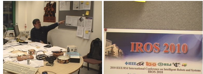
Fig. 1. A person points toward a specific region of interest. Due to the low resolution image, the content of the referred-to region can neither be reliably recognized nor learned. Using bottom-up saliency and the top-down information of the pointing gesture, it is possible to estimate the referred-to region. By foveating the region with a pan-tilt-zoom camera, an appropriate view for recognition and learning tasks can be acquired.
