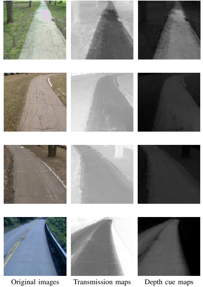
Fig. 2. Depth cue estimation results of some outdoor scene images in CMU/VASC image databases, which are selected from CMU/VASC image database: apr10-87-bright, jan25-91, jan31-91-down, july4-92-run6a, respectively.
