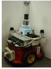
Fig. 1. The ActivMedia Pioneer P3-DX with two Hokuyo laser range finders and an omnidirectional vision system.
