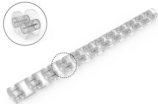
Fig. 3. 3-D rendering of robot assembly. Robot assembly is designed to feature 12 body segments, each of which contains two linear actuators. The detailed view of the body segment is shown on the left top corner.
