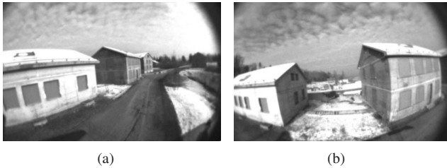
Fig. 7. The similarity between the buildings triggers some false positive loop closures. Here an example of false positive loop closure between nodes 1 and 17 in experiment 2.
