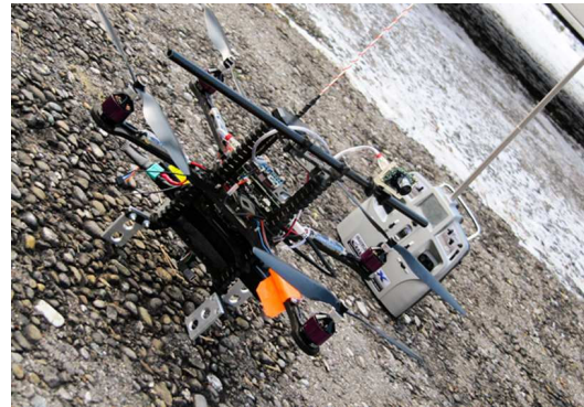
Fig. 1. Our robotic platform is a quad-rotor UAV.
