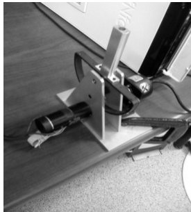
Fig. 3. Custom-made 1-DOF haptic device
