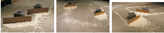
(c) Cooperative shoveling of the runway. (d) Splitting to two independent units. (e) Re-building of the formation.
