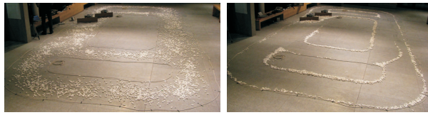
(a) Initial position of ploughs. (b) The ploughs have completed one cleaning cycle.
