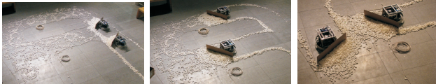
(f) Shoveling of the 2nd runway. (g) The formation is again splitted. (h) Beginning of the second splitting.
