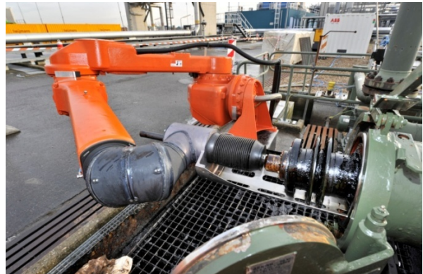
Figure 6 The robot performing its scraper handling task onsite.
