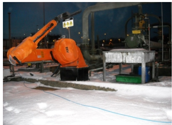
Figure 5 The ATEX certified ABB IRB5500 robot at the scraper station on a cold day during the demonstration period.
