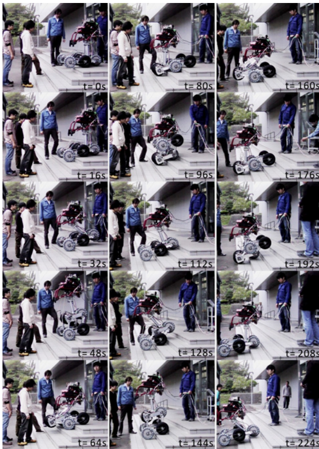
Fig. 9. Photos of the experiment descending stairs. (Riser height: 110 mm, tread depth: 300 mm)
