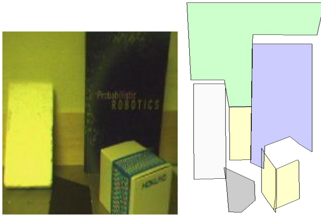
Fig. 6. 3D scene results: (left) 20° camera image. (right) 3D polygons.
