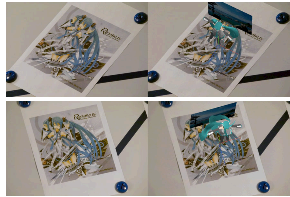
Fig. 22. examples of posture estimation results: input image (left) and superimposed image (right)
