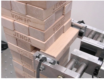
Fig. 12. Grasping side block to remove
