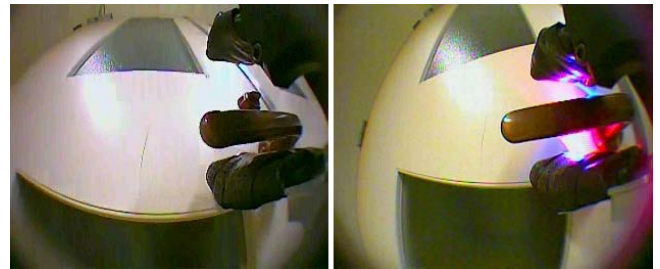
Fig. 9. Gripper camera view without LED(left), with LED(right)
