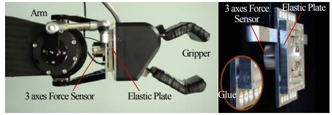
Fig. 6. Assembled force sensor and elastic plate
