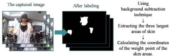
Fig.11. The image processing steps of extracting human motions.
