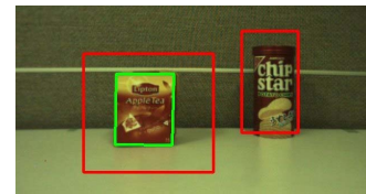
Fig. 2. Object recognition example: candidates (red) and recognized (green).
