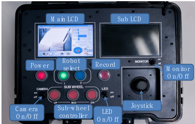
Fig. 5. Joystick-based remote controller
