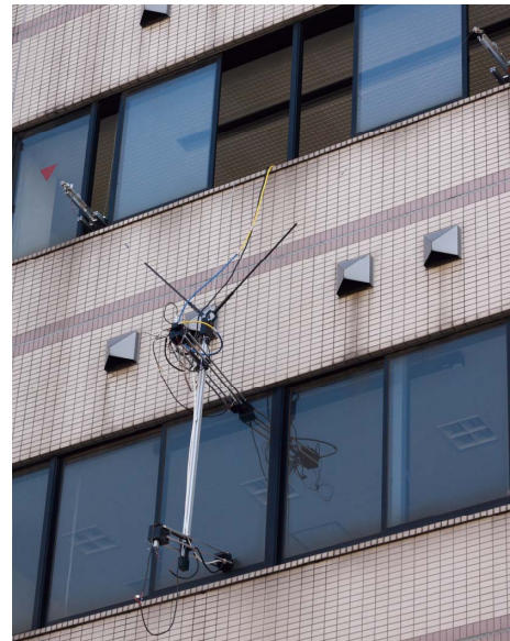
Fig. 1. Whole Windows Cleaning Robot “SkyScraper-I”.
