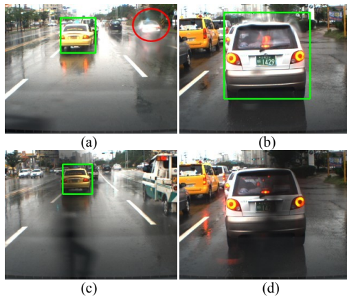
Fig. 14 Major factors that degrade the vehicle detection rate in rainy day (a, b) distortion caused by raindrops on the front windshield (c, d) occlusion by wipers
