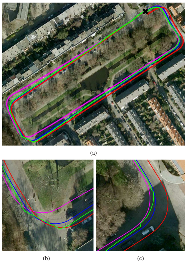
Fig. 3. Results on trajectory consisting of approx. 1200 poses estimated from binocular data, aerial image overlay (a), close-up of lower left corner (b), close-up of lower right corner (c). Binocular odometry (red), closed form algorithm (blue), ML solution (magenta) and differential GPS (green). The black cross depicts the loop-closing point.
