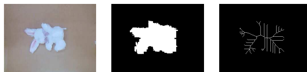
Fig. 3. LEFT: An isolated object to be classified. MIDDLE: The binary mask of the object. RIGHT: The image-based skeleton.
