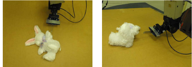
Fig. 1. The proposed setting for manipulation-guided sensing. The robotic system automatically learns the characteristics of an object by interacting with it. An overhead camera (not shown) is used for sensing the object.
