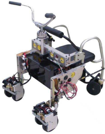
Fig. 1. The omnidirectional mobile robot in developing for the elderly's walking support and the caregiver's power assistance
