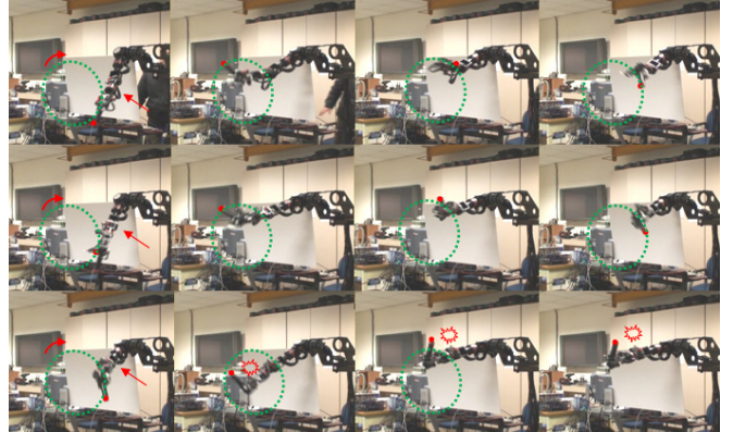
Fig. 7. Snapshots of the experimental results for the 7-DOF robotic arm with respect to the circular motion when sensory feedback of the neural oscillators was turned off.
