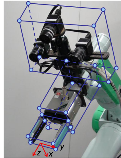
Fig. 7. Model of end-effector with three boxes
