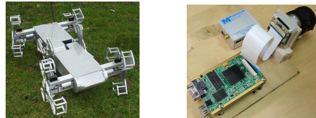
Fig. 1. The DAGSI Whegs Robot and Camera/IMU Setup.
