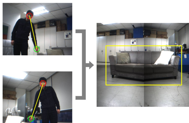
Fig. 4. Contacting two corner points of a sofa (large object) for multiple views; the robot captures four images and merges them into one
