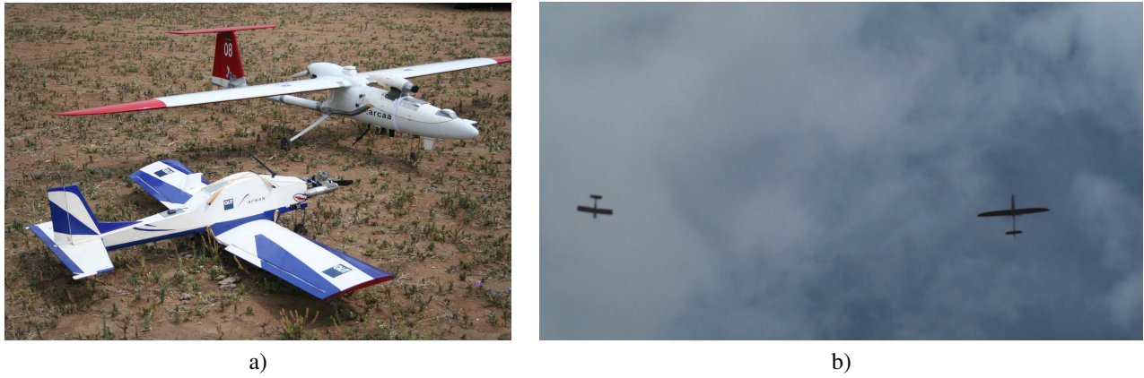
Fig. 2. Deployed UAV platforms for data collection. a) Flamingo UAV with camera pod (used as own aircraft) and boomerang (used as target). b) Actual moment of an encounter scenario showing both platforms
