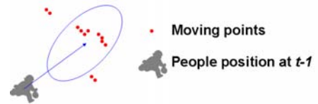
Fig. 4 Thresholds for classification of moving points in data association.
