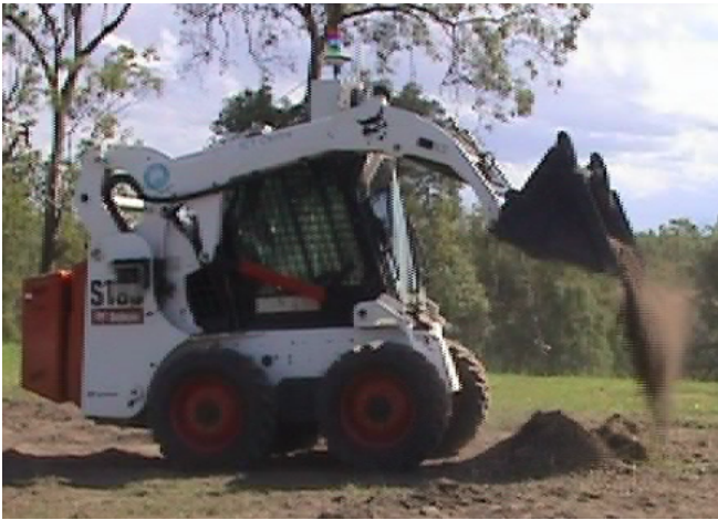
Fig. 2. Autonomous skid steer loader performing an earth moving task. Laser data from both the side lasers and top rotating laser scanner are combined into occupied voxel list maps based on various lattices.
