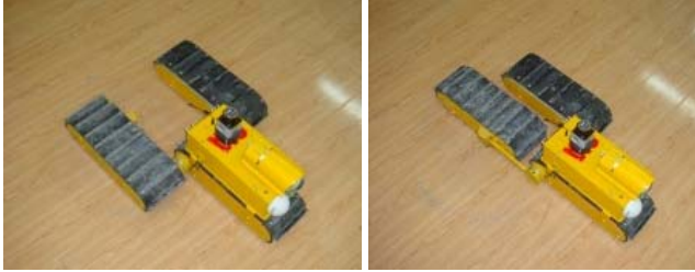
Fig. 2. Two representative configurations of the shape-shifting robot
