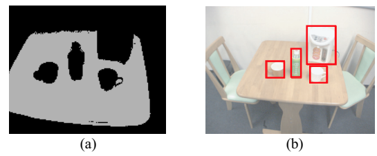
Fig. 8. Object detection based on plane detection. (a) Detected plane, and (b) Detected objects.
