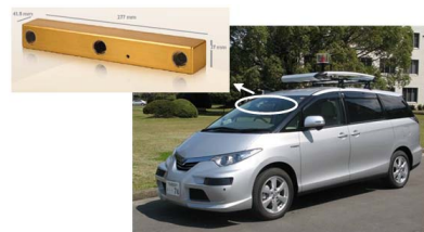
Figure 2. Our experimental intelligent vehicle and the stereo camera
