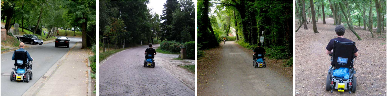
Fig. 2. The Bremen Autonomous Wheelchair Rolland driving along different roads during the experimental test runs. The particle filter explicitly models street widths for different classes of roads (cf. Table I). The roads above are classified as residential road, living street, path, and footway (left to right).
