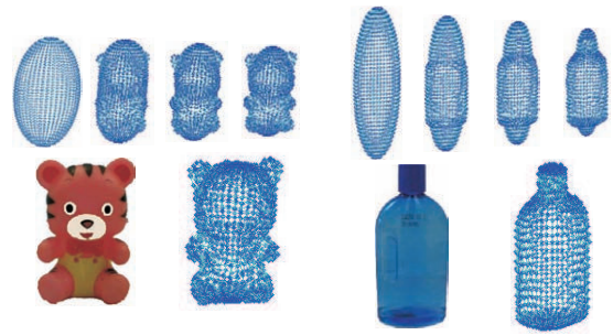
Fig. 6. Steps of the object surface reconstruction process.
