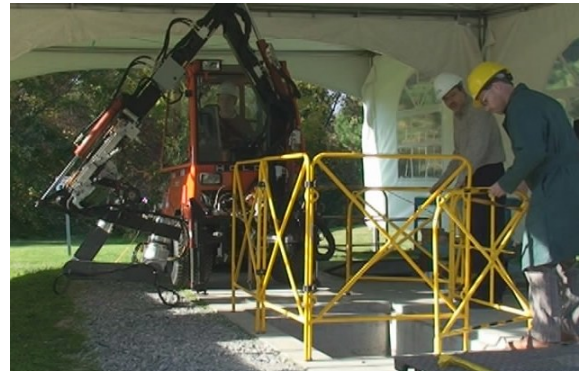
Fig. 5. Mobile robot prototype in operation in IREQ vault
