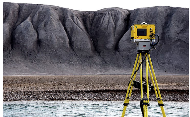
Fig. 2. Data for this study was collected with the Optech ILRIS3D-ER lidar. Long range lidar scans and panoramic images were collected in a planetary analogue setting on Devon Island, in the Canadian High Arctic.
