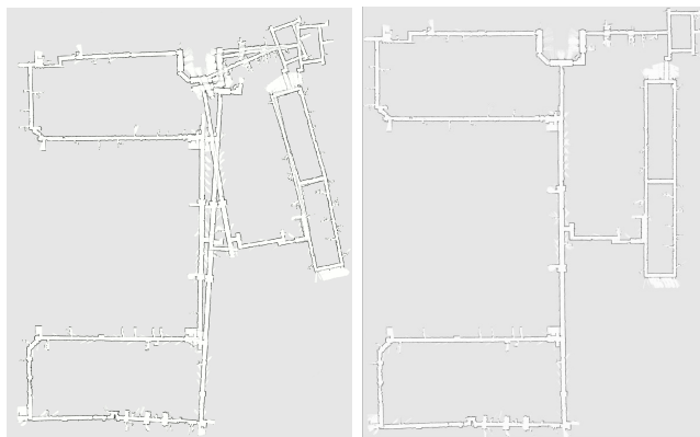
Fig. 1. Large MIT corridor map, unoptimized (left) and optimized (right). A full nonlinear optimization of this map (3603 nodes and 4986 constraints), starting from the odometry positions of the left-side figure, takes just 150 ms with our method.
