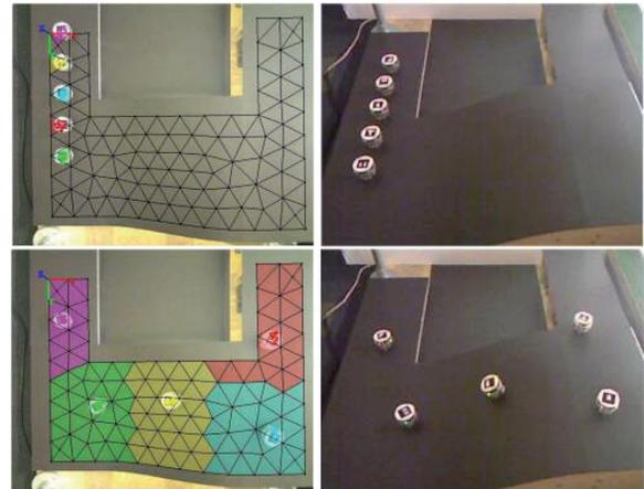
Fig. 1. Distributed coverage of a curved surface with hole. Five e-puck robots run Algorithm 2 and cover the non-planar non-convex surface (left: top view with surface mesh and Voronoi partition overlay, right: side view).
