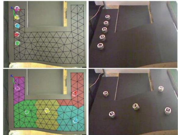
Fig. 1. Distributed coverage of a curved surface with hole. Five e-puck robots run Algorithm 2 and cover the non-planar non-convex surface (left: top view with surface mesh and Voronoi partition overlay, right: side view).
