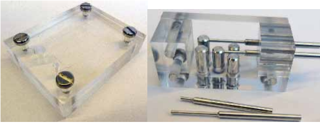
Fig. 3. Acrylic molds for tactile display fabrication.
