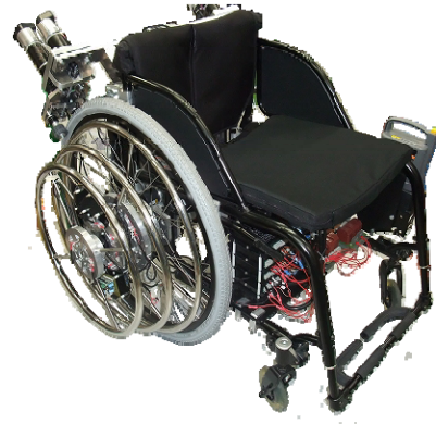
Fig.1. A prototype of one hand drive wheelchair with new assist units
