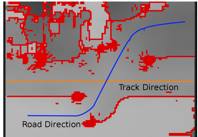
Fig. 5. Edges detected using the Robert's cross operator after removing noise. This intersection is the same as the one shown in Fig. 6. The road and track have been labeled manually for reference.
