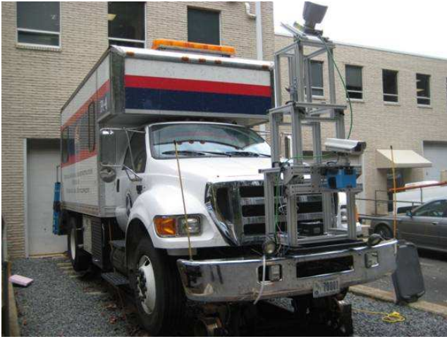
Fig. 2. Modified truck used for data gathering. The Velodyne HDL is mounted facing the ground at an angle to improve resolution of the ground surface immediately in front of the truck.
