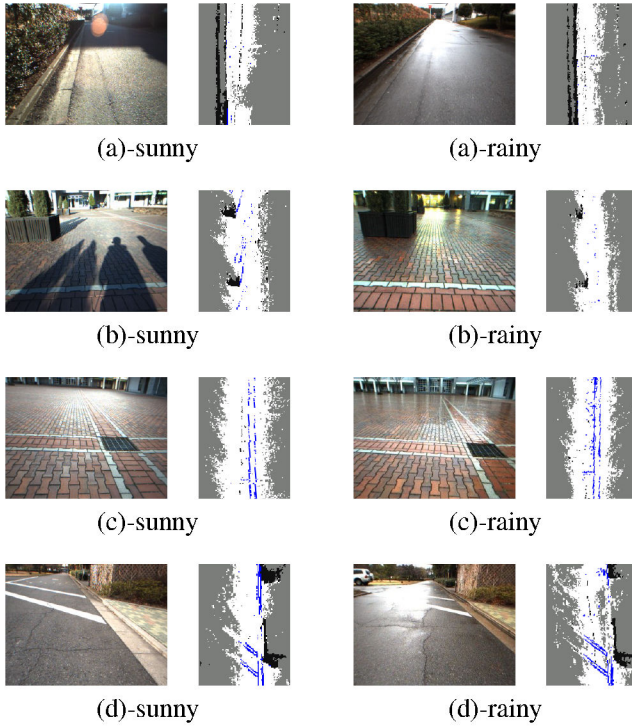
Fig. 5. Images and grid maps under various illumination conditions. Each row shows two sets of an image and a map of the same location obtained under sunny and rainy weather conditions. Colors in the maps indicate labels for cells: occupied (black), free (white), road landmarks (blue), unknown (gray).
