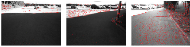
Fig. 11. Images obtained during experiment. Left: visual odometry not functional because of few edge points. Center: pole in the image used for visual odometry while turning to right. Right: camera exposure was adjusted to the shadow after turning.
