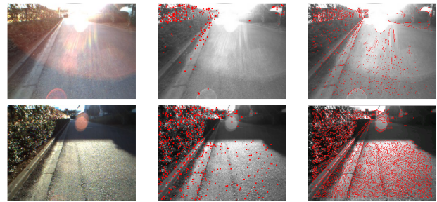
Fig. 1. Two images of the same place captured at different times and result of image feature detection. Left: original image. Center: Key points detected by SIFT. Right: Detected edge points. Lowe's SIFT Keypoint Detector [5] was used to detect the SIFT key points.
