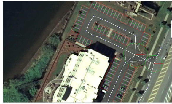
(b) Inaccurate segmentation results in extending the resulting lane-graph to the outside of the parking lot. There are 31 out of 430 local maxima used as vertices.
