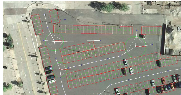
(d) There is an isolated vertex at the top left because of inaccurate segmentation. There are 35 out of 298 local maxima used.
