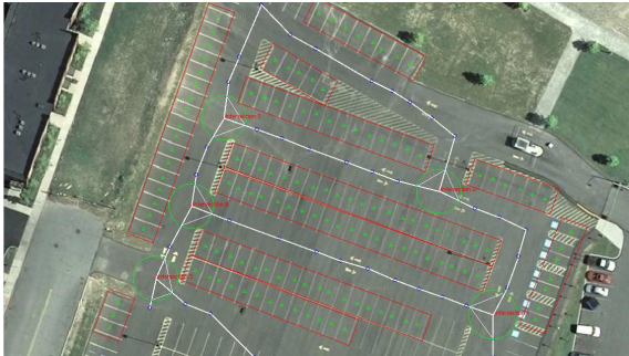
(c) Some of the parking spots at the bottom left are missed by the parking spot detection. This cause our algorithm to overestimate the actual parking lot area. There are 43 out of 428 local maxima used as vertices.
