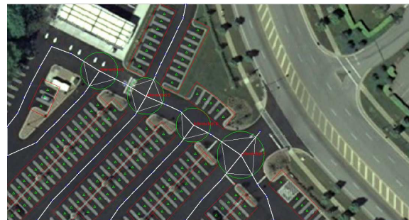
(f) The output of our lane-graph generation algorithm. A vertex is represented as an intersection if its edges are more than 2.
