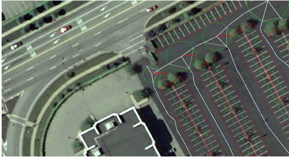
(a) The parking lot area is underestimated due to the shadows of trees. As a result, some edges of the resulting lane-graph do not align with the center-lines of drivable regions. There are only 37 (depicted as blue circle) out of 472 local maxima used as the vertices of the resulting lane-graph.
