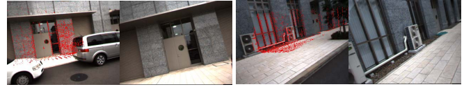
Fig. 9. 3D localization in outdoor environments. The red dots represent the 3D map reprojected onto the image.
