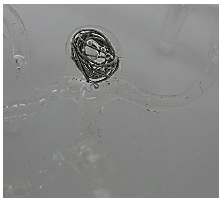
Fig. 19: Coil placement treatment simulation in silicone model of aneurysm.
