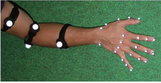
Fig. 2. Positions of the attached infrared reflection markers. We attached the marker on each joint to simplify estimating trajectories of joint angles.
