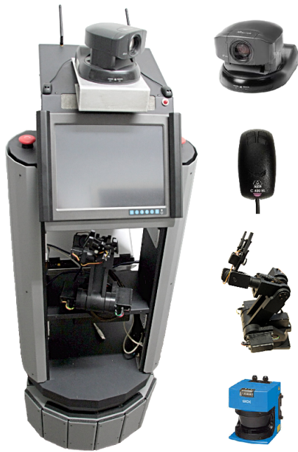
Fig. 1. The robot BIRON II with its hardware components shown on the right. From top right: Pan-Tilt-camera, interfacial microphone, Pioneer 5DOF arm, and laser range finder.
